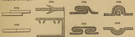
Fig. 4766 is the lap-joint without solder; it is set down flat with a steam-set, and used for smoke-pipes and other arrangements not required to be steam or water tight.
